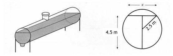
(a) Calculate *x*, the width (in metres) of the oil surface.
